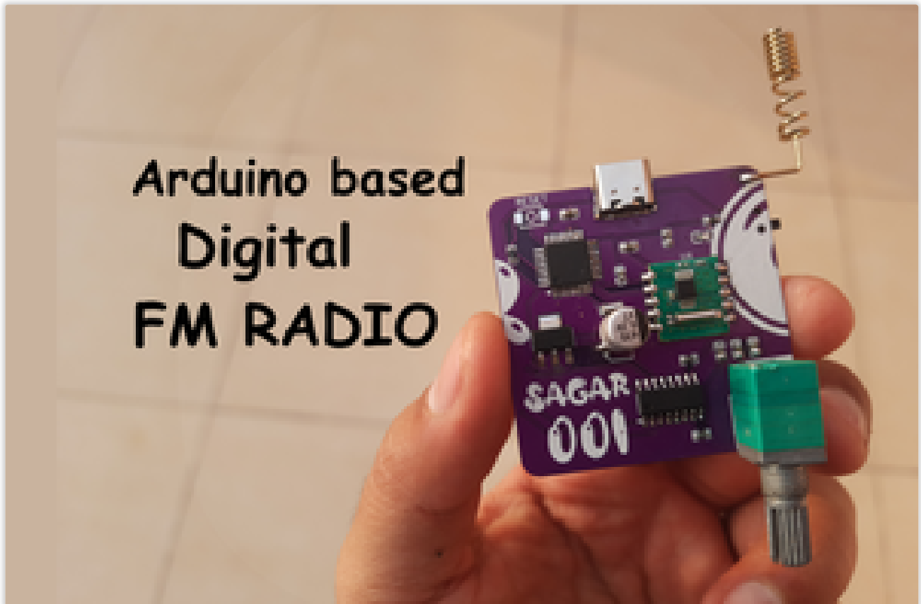
Arduino based Digital Audio FM Radio using RDA5807
